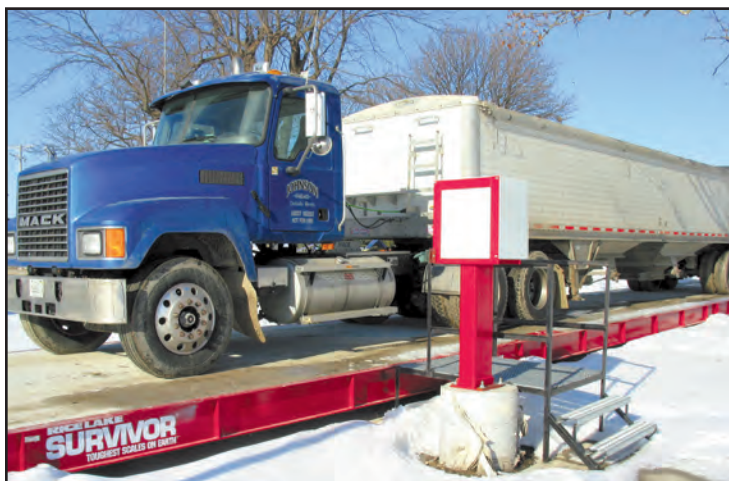
The 70-foot truck scale replaced a shorter scale that had been used at Johnson Farms for many years. This helps improve accuracy of weighing the contents of the truck since the entire load can be weighed all at once.
